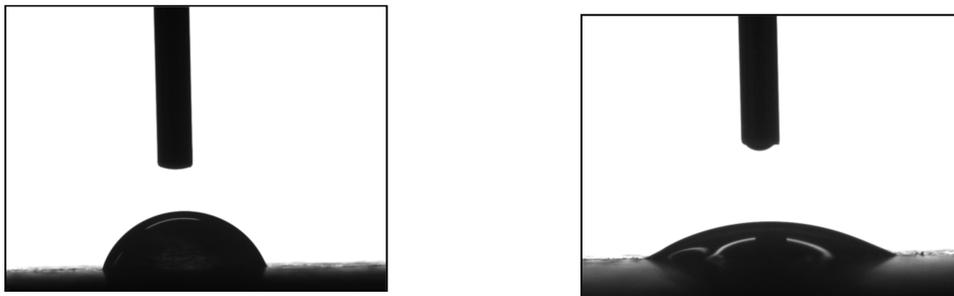
Fig.2 - Profile of the water drops at time 0 (image on the left) and at 76 hours (image on the right) on a Kreo White Active slab.
